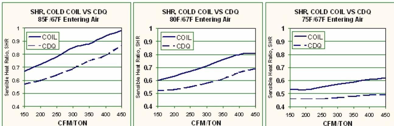
represented in terms of latent capacity improvement. The latent capacity improvement at the examples conditions range from 15 to 550 percent.
