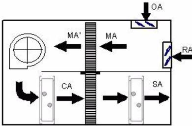
Most applications of the CDQ air handler will have components configured as described in the previous examples: outside air and return air inlets, filter, wheel pass one, supply fan, cooling coil, wheel pass two, then optional reheat coil.
