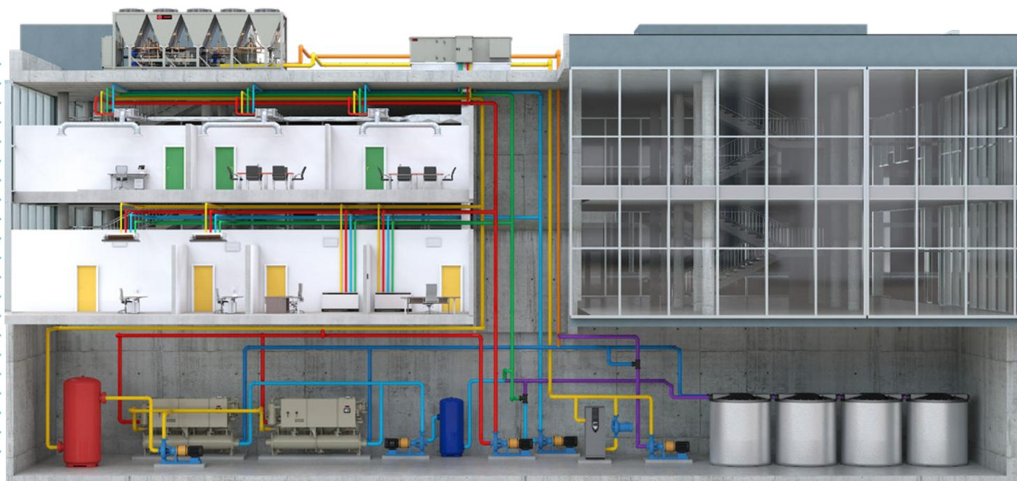
Trane's SSHP system uses thermal energy storage tanks to increase the usefulness of TES, as well as the air-to-water heat pumps.
